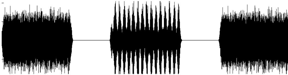
Figure 1: The unmodulated noise signals (left and right) and the modulated noise signal (middle)
