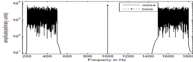
Figure 3: Spectrum of notched noise centered at 1000 Hz with  $g = 0.5$  along with the 1000 Hz probe tone.
